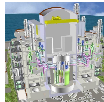
Tank-type sodium-cooled fast reactor ( https://www.mhi.com/news/23071202.html )
